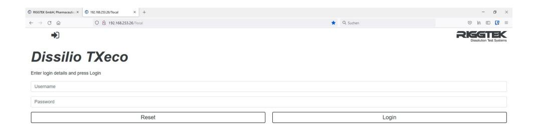
If the Dissilio is connected to your local PC or your company network, simply enter the IP-address of your Dissilio in your (Internet)-Browser to reach the Login-Screen – as shown above. If you have several Dissilios, you can easily connect to several Dissilios at the same time, having one Dissilio in each Browser tab.
