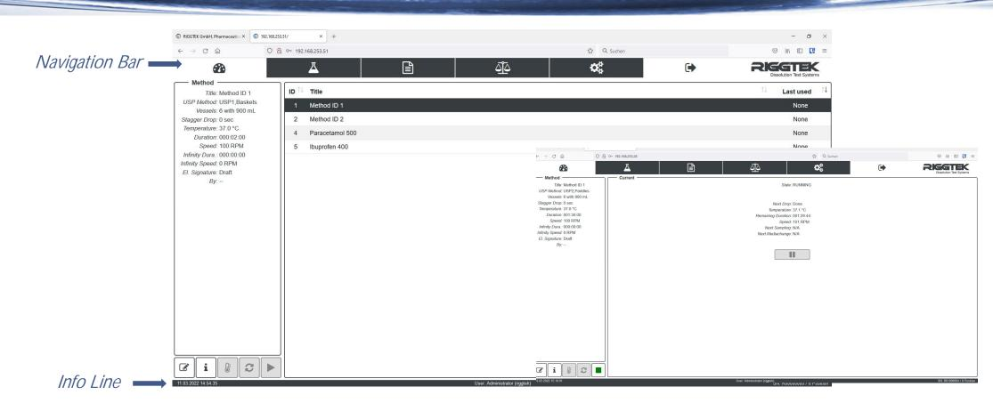
After the successful login, the "Dashboard" will appear. The Dashboard allows you to overview easily existing methods or the actual status / live monitoring of a running method - remotely with your PC. At each screen you find the Navigation Bar at the top and the Info Line at the bottom, showing you the serial number of the Dissilio, date and time and the user logged in with which permission role.
