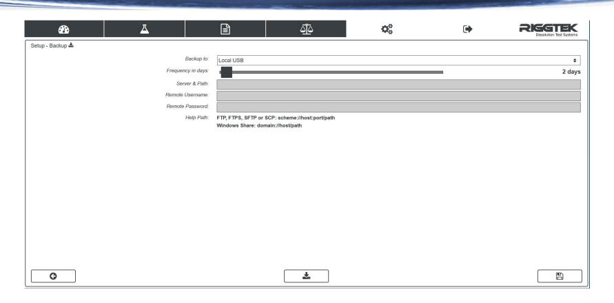
The optional "Backup-Package" \* allows to make backups of the whole system to USB, Windows-Shares, FTP-, FTPS-, SFTP- or SCP-Server. The backup can be done manually or automatically.
