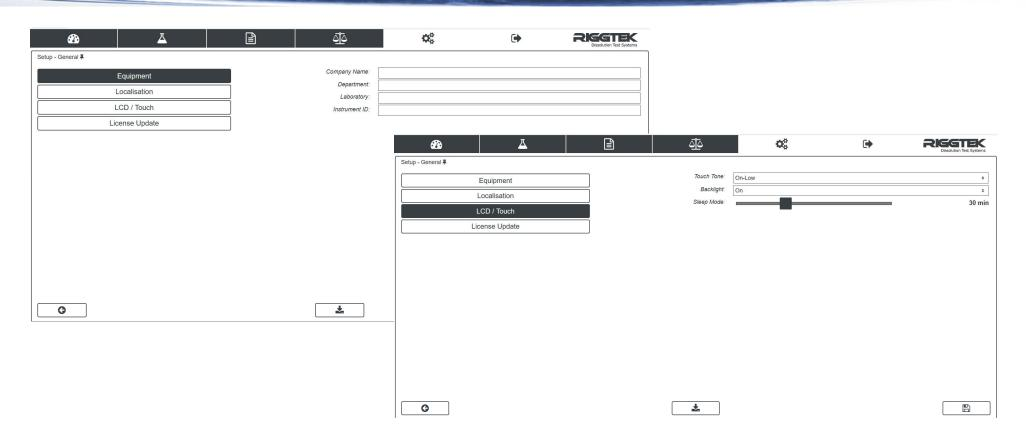
The "Setup-General" tab allows to easily personalize your Dissilio with e.g. an internal Instrument-ID, Company name etc.
