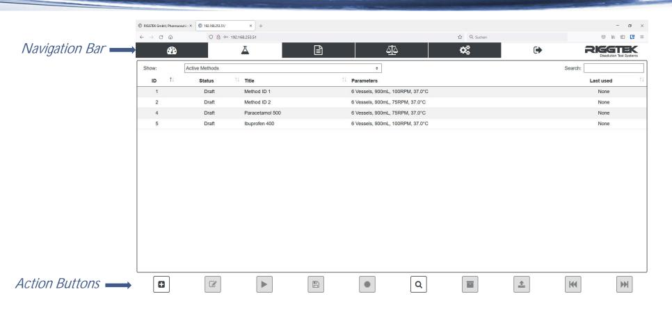
In the "Method Menu" methods can be easily found, added, edited, printed, electronically signed or archived with the action buttons. Sorting by colums and a free text search are helping to easily find the right method. With the optional TOP-Package\*, methods from a "Parent-Dissilio" can be easily imported to have easily the same methods on several Dissilios.
