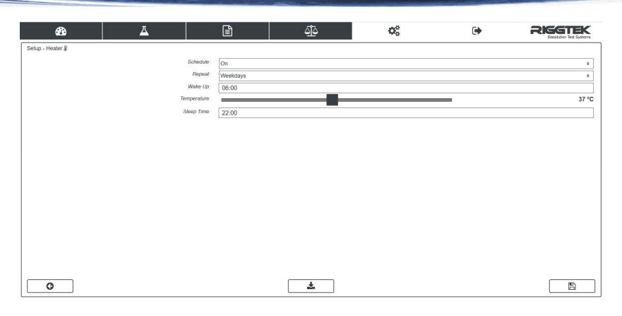
In the "Heater"\* (part of optional ENERGY-LIGHT-Package\*) tab the wake-up and sleep time can be edited via your PC using the Browser Interface. These settings can be changed easily remotely when shifts are changing or a holiday season is coming without going to the individual Dissilio. This allows to save considerably much energy without loosing time for heating up the waterbath.
